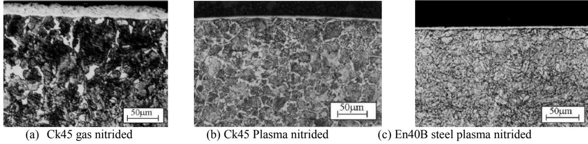
Fig. 1. Optical micrographs of typical nitrided specimens.
