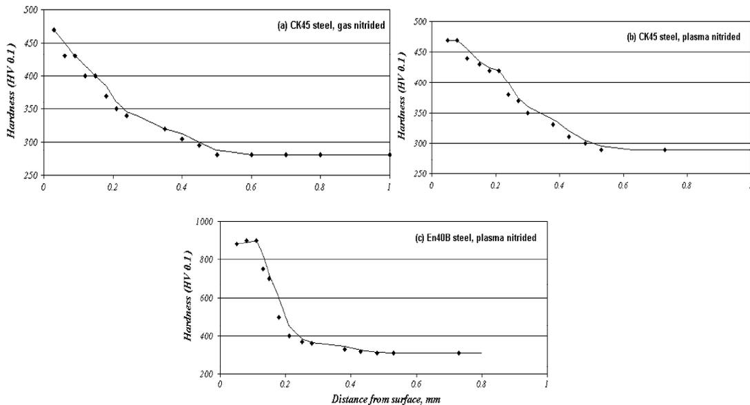
Fig. 3. Hardness gradients of nitrided specimens
