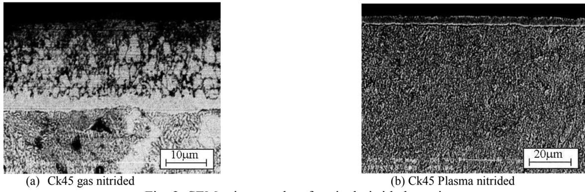
Fig. 2. SEM micrographs of typical nitrided specimens.
